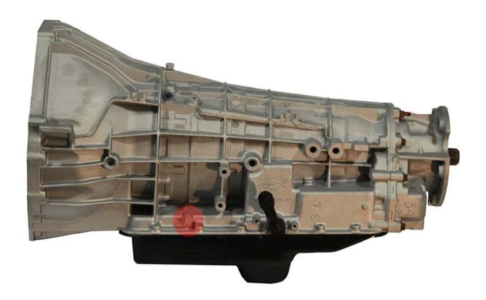
If your truck is a manual transmission and you want to run the Transmission Temperature Sensor, you will need to fabricate something for the sensor to mount in the transmission fluid, such as in the face of the PTO cover on a ZF6.
